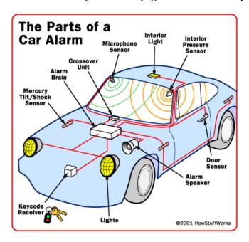
Only the siren (alarm speaker) will be disconnected when the ban goes into effect. A qualified installer can shut off the siren and install a replacement pager in under one hour. There are several add-on pagers available from most installation shops. Source: Tom Harris, "How Car Alarms Work", http://www.howstuffworks.com/car-alarm.htm
