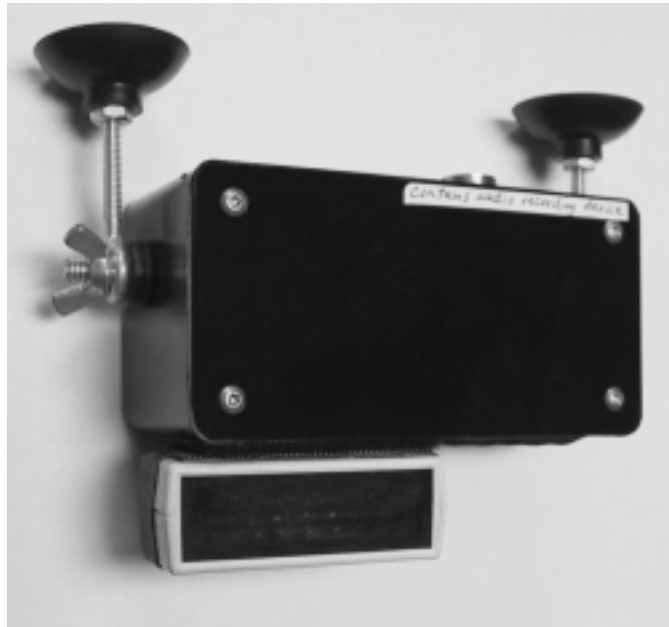
Figure 3. Photo of exterior of camera unit.
